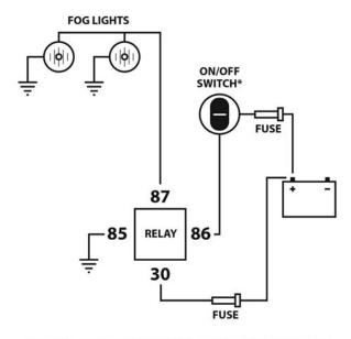
\*As an alternative, instead of running directly from the positive terminal to the fog lights' on/off switch, run power from the headlights after the headlight switch to the fog lights' on/off switch so the fog lights will not go on unless the headlights are on.
